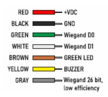
Wiegand 27-66 bit Wiring Diagram
