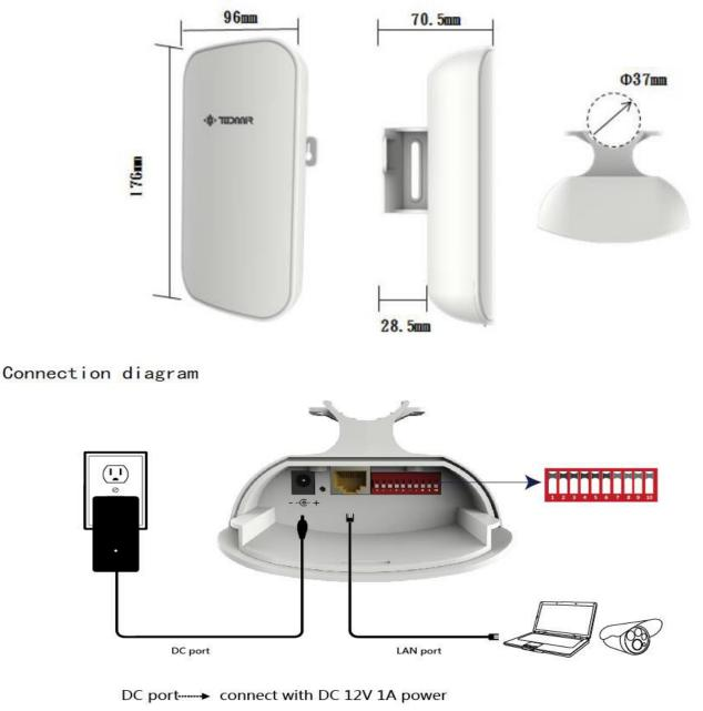
LAN port ------>connect with pc, camera, switcher, NVR
