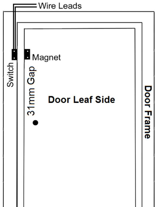
1. Place the switch (with wire) on door frame, mark the mounting position and fix the screw in door frame to mount the switch
