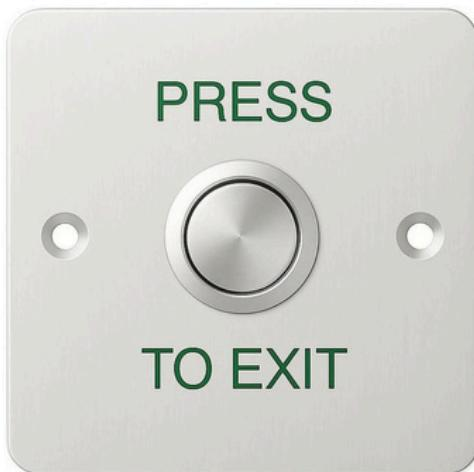
The DA-ELEB3W Waterproof Press Exit Button is built with a robust 304 stainless steel panel, offering excellent durability for both indoor and outdoor applications. With a contact rating of 8A at 125V AC and 5A at 250V AC, it provides reliable performance under various electrical loads.
